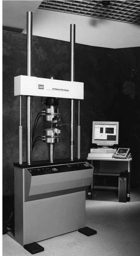
Figure 2.1 Tensile loading machine with automatic data-processing system. (Courtesy of MTS Systems Corp.)
